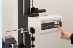
Centralized front control panel
